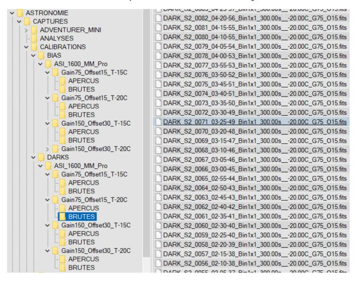
The raw images are sorted by calibration type (offset or dark), by sensor, then by camera gain, camera offset and temperature. Each series of raw images is stored in a "RAW" directory and the associated "quick look" images in an "PREVIEW" directory.
